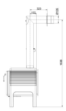
... with horizontal smoke pipe connection kit L form
