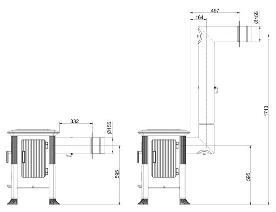
... with horizontal smoke pipe connection kit and Z
